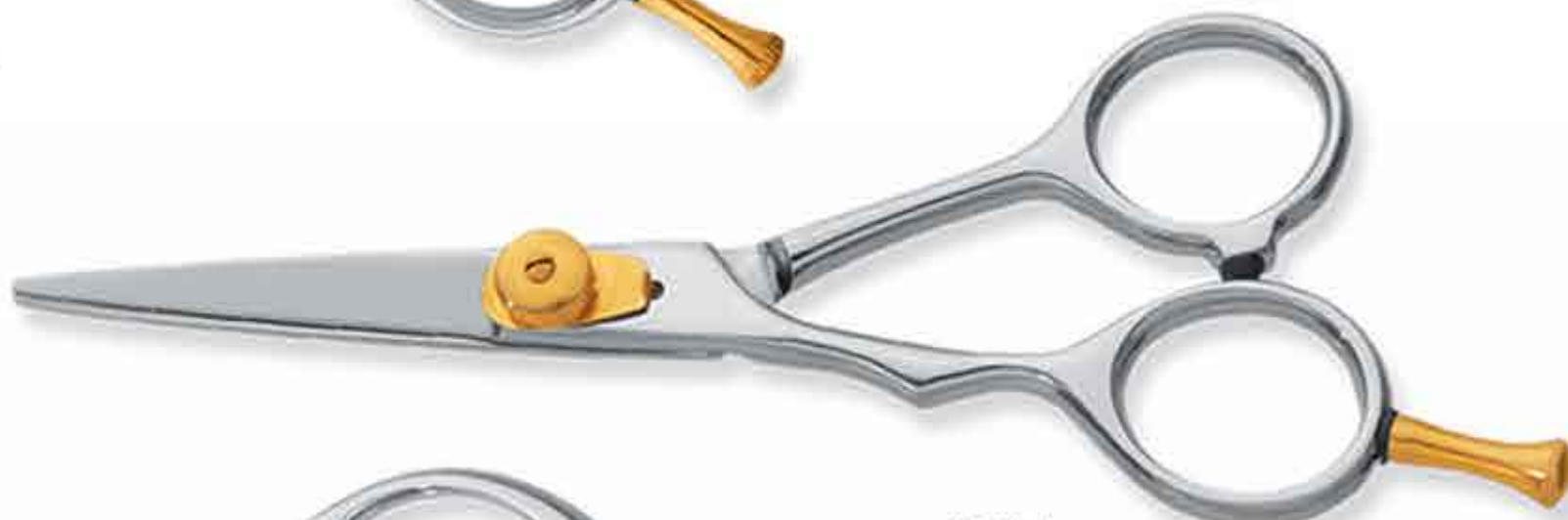
0-004 Sizes: 4.5", 5.0", 5.5", 6.0", 6.5", 7.0" Hand-made two piece style. Hollow-ground blades. Removable Trumpet finger rest. Leaf spring tension screw system.
